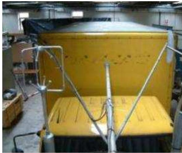
Figure 6: Front view. Front tapping points, anemometer
