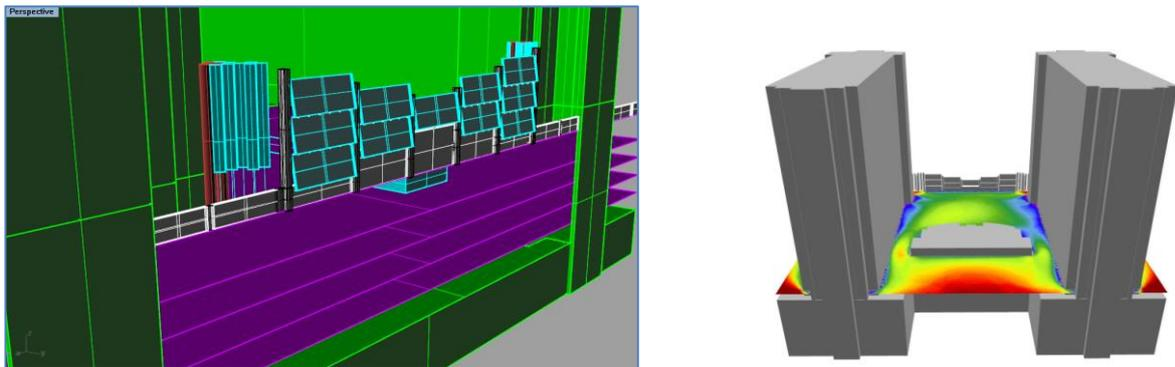
Figure 6. Original Windbreak Design and Wind Comfort index at the pool level
