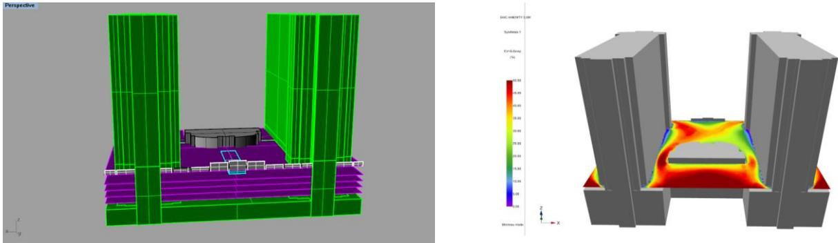
Figure 5. Original Windbreak Design and Wind Comfort index at the pool level
