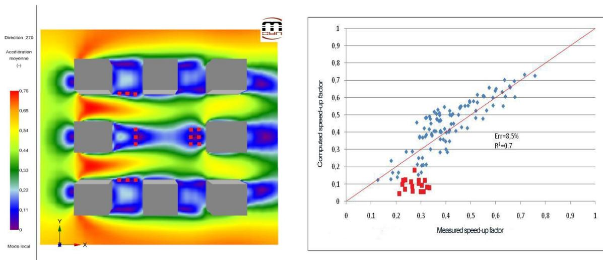
Figure 2. Wind flow around the blocks (wind from left to right) and computed vs measured normalized wind speeds.
