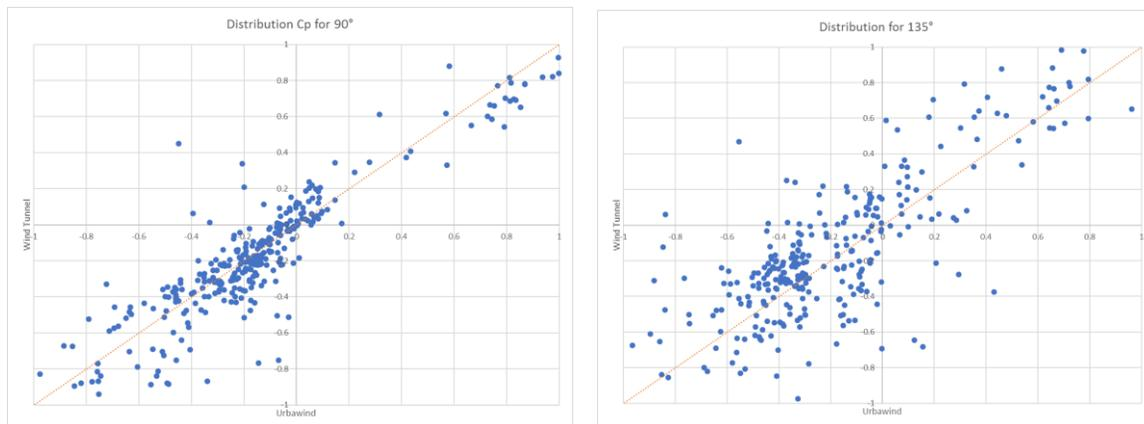
Figure 2 – Correlation factor between wind tunnel and simulation results for 90° (=0.90) and 135° (=0.79)
