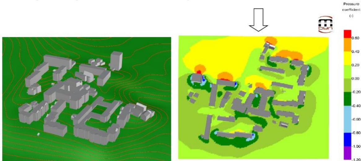
Figure 1 – CAD of the project and example of wind computation map (Pressure coefficient)
