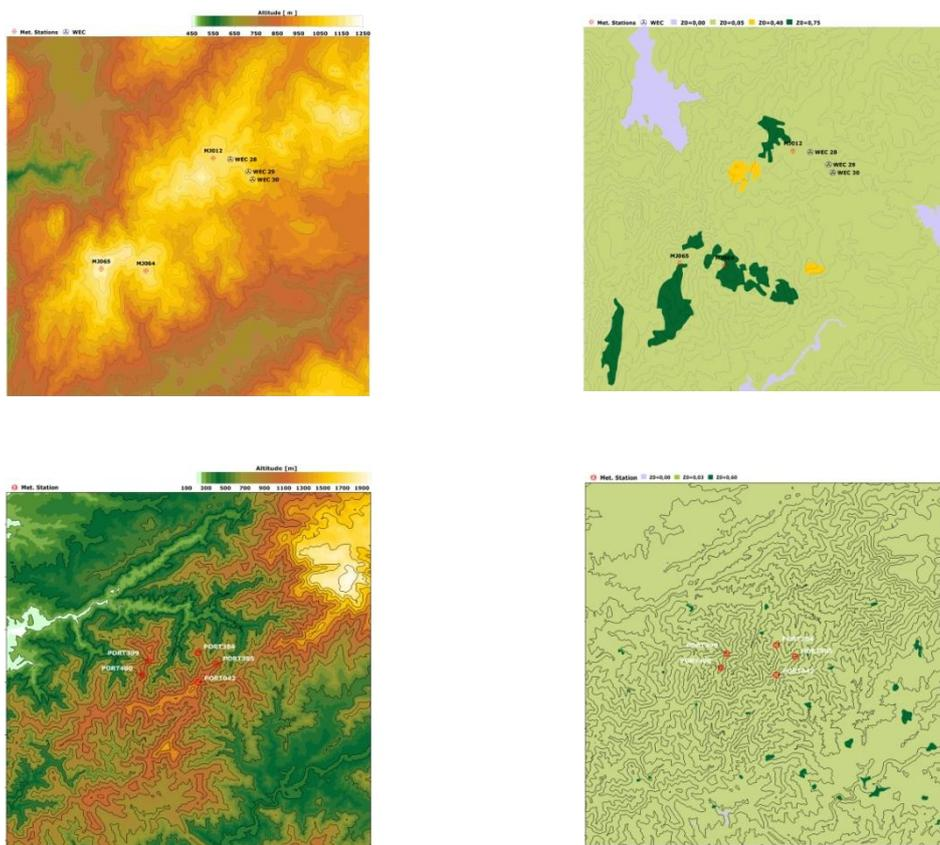
Figure 2 - Example of altitude and roughness length maps used
