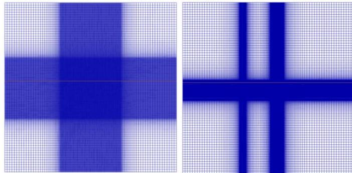
Figure 4 - Example of a horizontal expansion of a calculation mesh, 50m, at left and discrete points, 25m, at right
