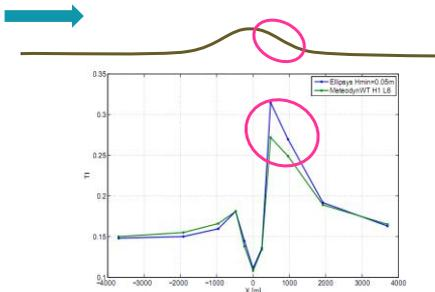
Figure 4.31.: Turbulence intensity horizontal profiles. Moderately steep Gaussian hill, simulated on MeteodynWT and EllipSys with the finest meshes; at 40m above ground
