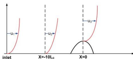
Figure 4.4.: Definition of the wind speed for the speed-up calculation with WAsP
