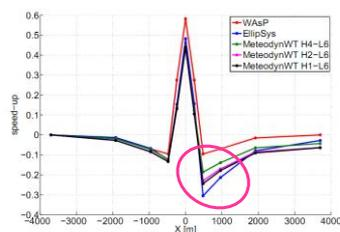
Figure 4.24.: Horizontal speed-up profiles. Moderately steep Gaussian hill, simulated on MeteodynWT and EllipSys with the finest meshes; at 40m above ground
