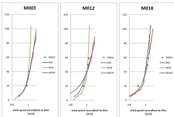
**M003:** free stream direction. Roughness tuning needed in the WM.
