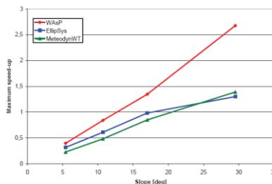
Figure 4.20.: Maximum speed-up at the top versus the hill's slope
