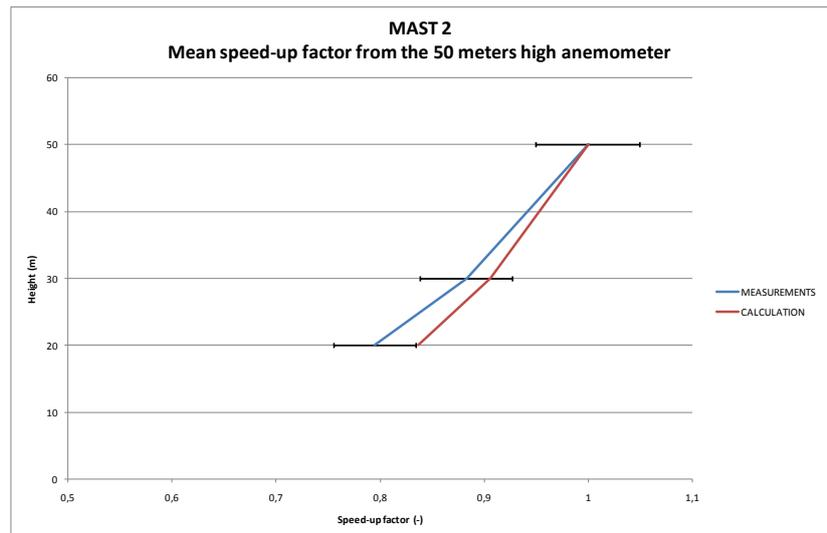
Figure 9: Error on mean speed up factor
