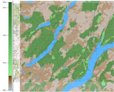
Figure 3: Roughness map derived from CORINE Land Cover 2000 database
