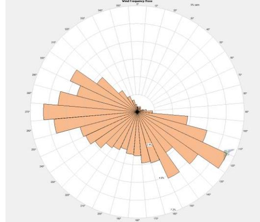
Figure 6: Wind rose at met mast 1
