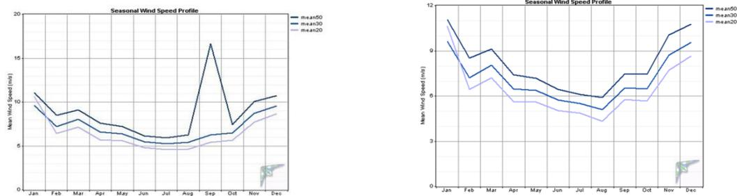
Figure 7: Monthly mean wind speed before (left side) and after (right side) the data correction
