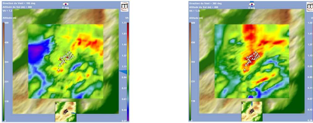
Figure 8: Speed up factor at 55 meters high for 100° (left side) and 360° (right side)
