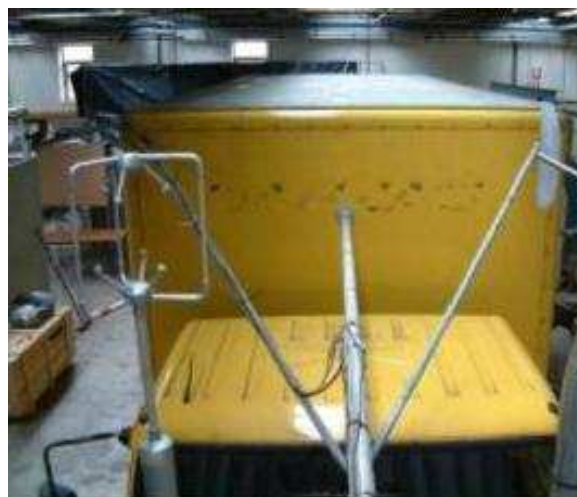
Figure 6: Front view. Front tapping points, anemometer
