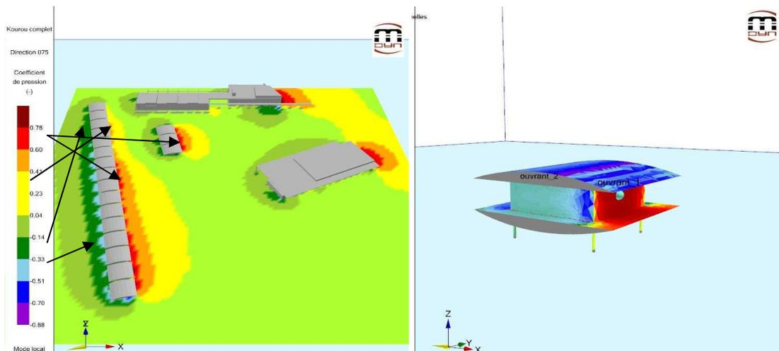
Figure 5: View of the secondary school and pressure coefficient field on an horizontal plane 4 meters above the ground (left) and on the walls of a classroom (right)
