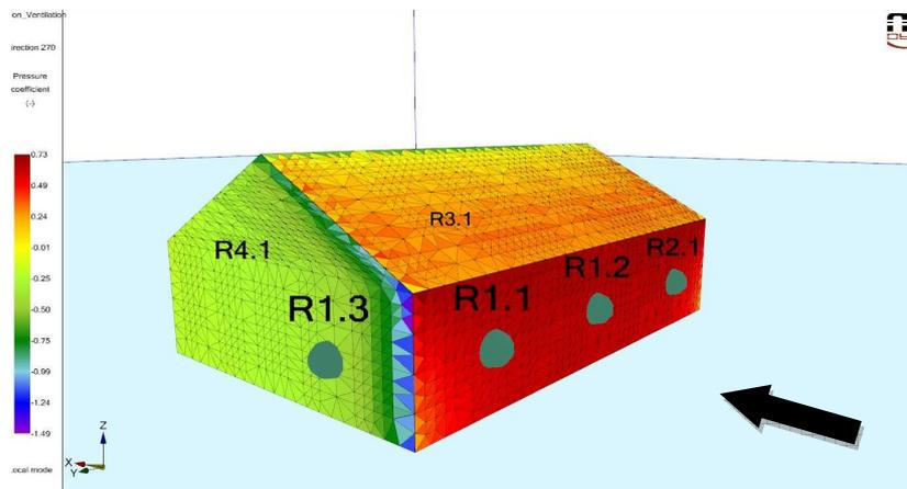
Figure 1: Pressure field on the façades and roof of a detached individual house. Openings are represented in grey.
