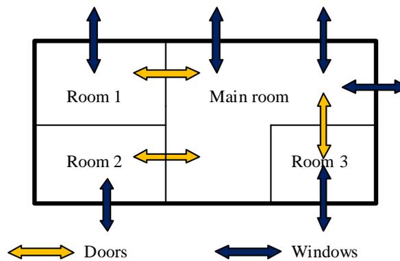
Figure 2: Openings (doors and windows) of the detached house
