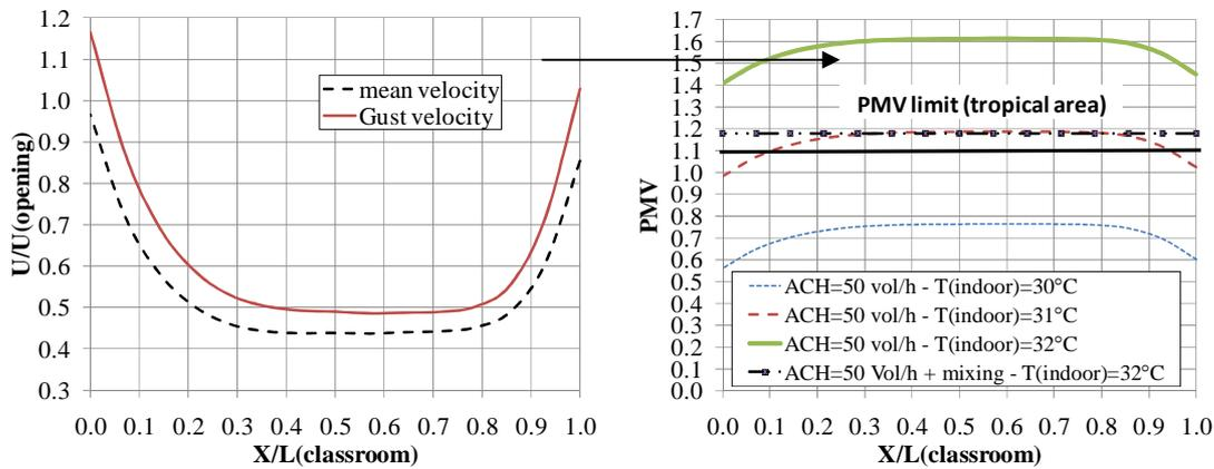
Figure 7: velocity on the center line between the inlet and outlet openings - PMV index in the classroom
