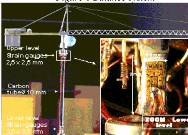
The two stages are connected by a 10mm diameter carbon tube that simulates the drag properties of the mast. The junction between the mast and the rotating part is adjusted using a central pin to reduce friction coefficient.
