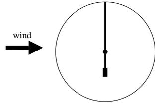
$$\overline{M}_{\text{resultant}}(\text{O}) \cdot \vec{y} = -\ddot{\theta} m_{\text{RP}} l_{\text{Mast}} - a(m_{\text{Mast}} + m_{\text{RP}})g + l_{\text{CP}} F_{\text{X}_{\text{Wind} \rightarrow \text{Mast}}} + l_{\text{Mast}} F_{\text{X}_{\text{Wind} \rightarrow \text{RP}}} \quad (4)$$
