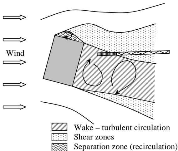
The presence of the building modifies the flow properties around the crane which can be then in various disrupted layers of circulation (Fig 2). These areas depend on the building sizes and turbulent scales of the oncoming wind. The instability properties of each zone can be noted. The wake zone can be characterized by low wind velocities and strong direction fluctuations induced by the vortices. In the shear layers, wind speed and in the same way aerodynamic loads increase.
