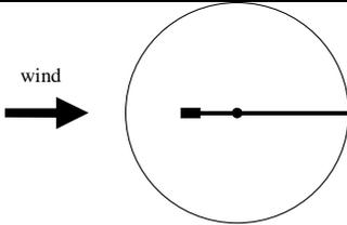
$$\overline{M}_{\text{resultant}}(\text{O}) \cdot \vec{y} = -\dot{\theta}^2 m_{\text{RP}} l_{\text{Mast}} r - a(m_{\text{Mast}} + m_{\text{RP}})g - r m_{\text{RP}} g + l_{\text{CP}} F_{\text{X}_{\text{Wind} \rightarrow \text{Mast}}} + l_{\text{Mast}} F_{\text{X}_{\text{Wind} \rightarrow \text{RP}}} \quad (2)$$
