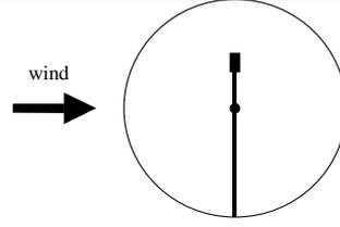
$$\overline{M}_{\text{resultant}}(\text{O}) \cdot \vec{y} = +\ddot{\theta} m_{\text{RP}} l_{\text{Mast}} - a(m_{\text{Mast}} + m_{\text{RP}})g + l_{\text{CP}} F_{\text{X}_{\text{Wind} \rightarrow \text{Mast}}} + l_{\text{Mast}} F_{\text{X}_{\text{Wind} \rightarrow \text{RP}}} \quad (3)$$
