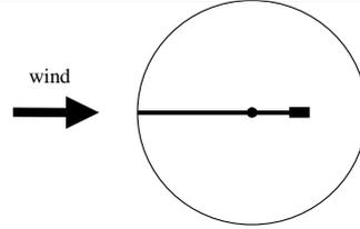
$$\overline{M}_{\text{resultant}}(\text{O}) \cdot \vec{y} = \dot{\theta}^2 m_{\text{RP}} l_{\text{Mast}} r - a(m_{\text{Mast}} + m_{\text{RP}})g - r m_{\text{RP}} g + l_{\text{CP}} F_{\text{X}_{\text{Wind} \rightarrow \text{Mast}}} + l_{\text{Mast}} F_{\text{X}_{\text{Wind} \rightarrow \text{RP}}} \quad (5)$$
