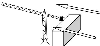
Figure 4 Rotating part longer than transversal dimension of the building
