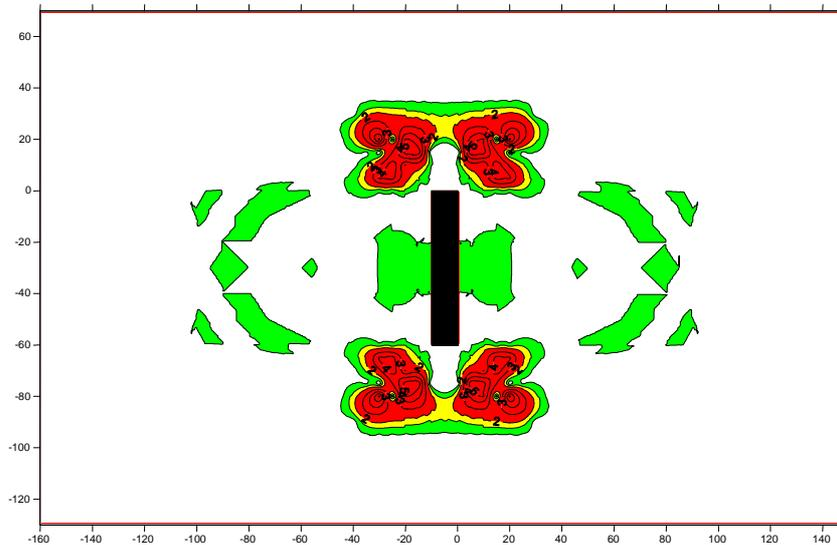
The Figure 12 shows an example of mapping. The crane was situated near a 48m high, 60m long and 15m large building. The jib height was fixed to 52m and the jib length to 45m. The critical locations are indicated in red. In this configuration, the environment effect is similar to a corner effect described in 5.1. The parametric study is in progress.
