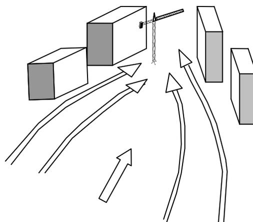
The local acceleration effects are more difficult to describe and to schematize. Indeed, several buildings interfere and there is not a simple schema to summarize all the configurations. The built environment creates a corridor where the wind is guided and accelerated in restricted areas. In general, the jib don't move and stay in a stable position but the aerodynamic loads increase. A typical example is the "Venturi" effect.
