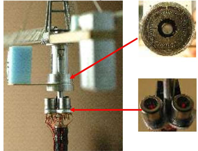
An angular encoder composed by three optoelectronics sensors and a reflecting surface provides the instantaneous angular position of the jib.
