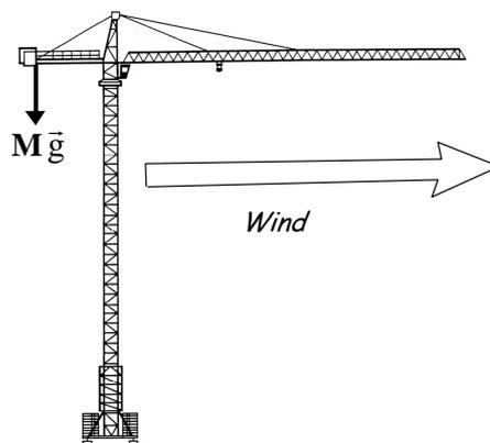
Without surrounding environment, the crane is in tail wind condition. The jib fluctuates and the counter weights of the jib equilibrate the aerodynamic loads.
