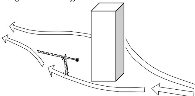
An upstream crane can be sucked in the lateral flow turning around the building. Then, it takes a
